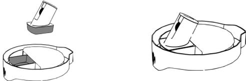
To fit the **valve**, turn the **lid** over and insert the **valve** into the recess provided. Press firmly until the retaining tabs snap into place on the right and left with a click.
